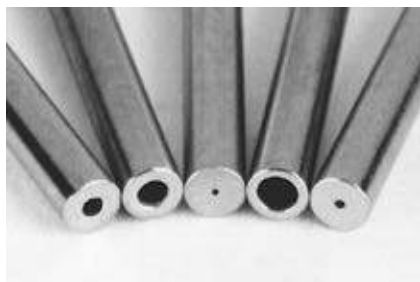
Electrolytically cut and polished
