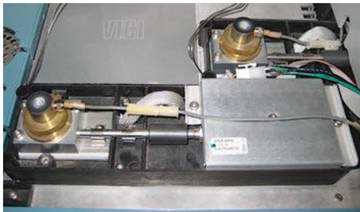
View of relocated Agilent FID to permit use of fast GC column kit
