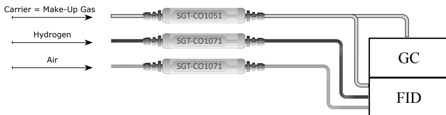
GC/FID Solution 1 (Carrier Gas = Make-Up Gas)
