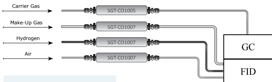
GC/FID Solution 2 (Carrier Gas differs from Make-Up Gas)
